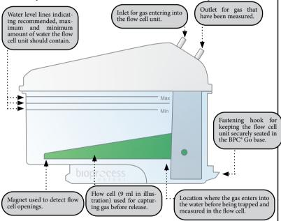
IMPORTANT: The flow cell unit (FCU) can NOT be opened. Any attempt to do so will risk damaging it and ruining the gas tightness. Also, always remember to use the apropriate calibration cell volume (configurable in the web UI) associated with each FCU.
